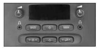
If your vehicle has the rear seat audio system, the lower buttons are used to adjust the rear seat climate controls. The temperature of the air coming through the rear outlets is determined by the front passenger's temperature setting.
